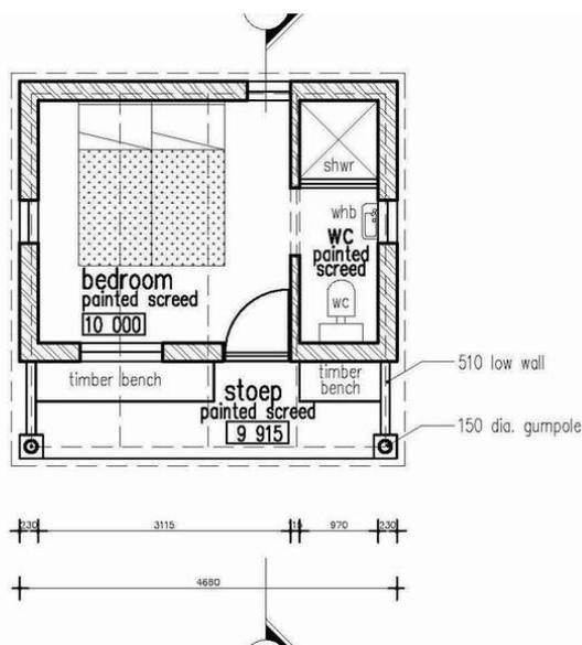
The floor plan for the guest room. The 2<sup>nd</sup> Phase of the development includes 20 overnight rooms and sewer plant. Construction of the first 3 rooms will start soon
